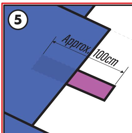
5. **IMPORTANT!** When a roof is built in several sections, each transition between two sections must include 100 cm Controlit connection stripes placed every 15 meters with at least **two** stripes used. This ensures electrical continuity across the entire roof.
