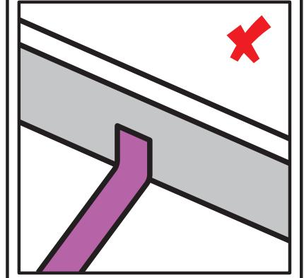
3. Controlit connection stripes must be rolled on horizontal surface only
