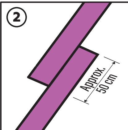
2. When you need to connect new roll of connection stripe, align it next to the other with an indent of 50 cm.
