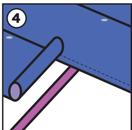
4. **IMPORTANT!** Connection stripes must always be placed perpendicular to the direction of the Controlit as shown in visualisation.
