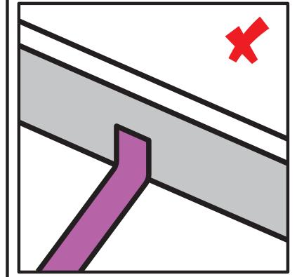
3. Controlit connection stripes must be rolled on horizontal surface only
