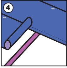
4. **IMPORTANT!** Connection stripes must always be placed perpendicular to the direction of the Controlit as shown in visaulisation.
