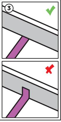
3. Controlit connection stripes must be rolled on horizontal surface only Controlit connection stripes **are not applied on vertical surfaces!**
