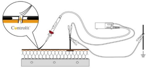
On the surface on the roof system, which must be dry, a direct current voltage, calculated according to the thickness of the waterproofing material (Dielectric Strength), is applied with brush of determined width, connected to the central unit,
